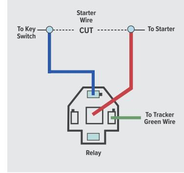
1. With a Voltmeter, find the wire from the key that activates the starter.
