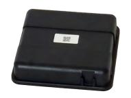
The MTM502 will be delivered in "Sleep" mode which is the lowest power state until the activation magnet is removed.
